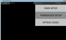
Here you can select the Transducer menu and by clicking on the transducer connector port you can move the transducer to the appropriate area of the vessel, and select the transducer, by part number. This will change the parameters to match your transducer.
