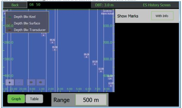
By selecting table, the depth of at least every minute and marks in between (indicating changes or highlighted events such as alarms or auto changes) are listed with time and position, if available.
